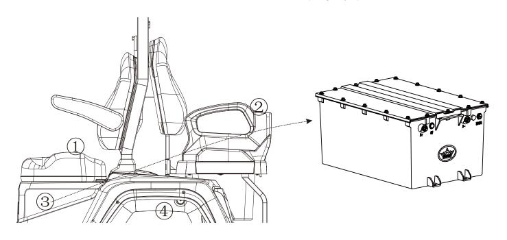
①LUXURY SEAT WITH FOLDABLE ARMREST ②REAR SEAT ARMREST WITH CUP HOLDERS ③LITHIUM BATTERY PACK .LONG RANGE 110AH(EXTENED RANGE 205AH OPTIONAL) ④AUTOMOTIVE E-COAT CHASSIS
