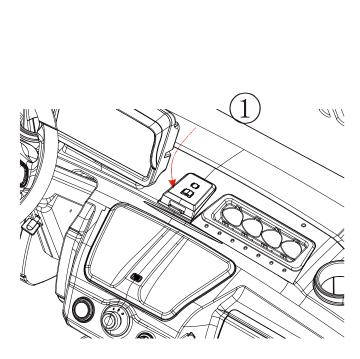
1.REMOVE THE BRAKE OIL POT COVER ON THE DASHBOARD TO GET ACCESS TO THE OIL TANK.
