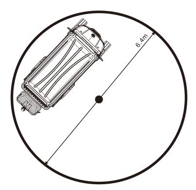
**Vehicle Turning Clearance Diameter**
