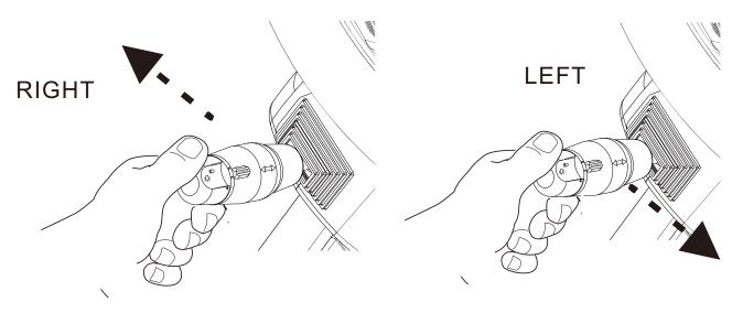
PUSH & PULL THE CONTROL STALK FORWARDS OR BACKWARDS TO ENABLE LEFT TURN SIGNALS OR RIGHT TURN SIGNALS.
