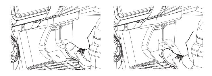
1. USE ACCELERATOR PEDAL TO ACCELERATE 2.APPLY BRAKE PEDAL TO REDUCE SPEED
