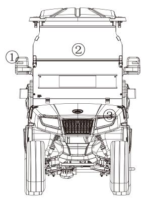
①REARVIEW MIRRORS WITH TURN SIGNAL INDICATORS ②FOLDABLE WINDSHIELD WITH SILDABLE AIR VENTS ③HEADLIGHTS
