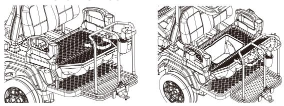
1.FLIP THE REAR SEAT UP. 2.REMOVE THE STORAGE BUCKET COVER.
