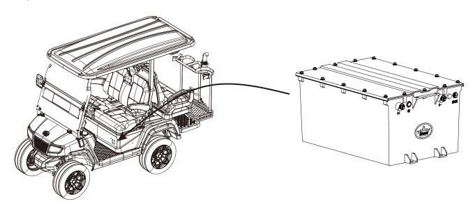
The lithium iron phosphate battery (LiFePO4 or LFP) is the safest of the mainstream lithium battery types. A single LFP cell has a nominal voltage of 3.2V.
