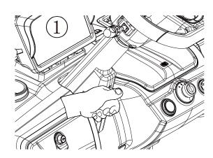
1.PRESS THE ADJUSTMENT KNOB SHOWN IN PIC 1 DOWNWARD.
