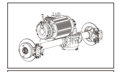
Check the brake shoes worn out conditions, if it is extremely worn out(1/3 left), then the brake shoes need to be replaced with a new one.
